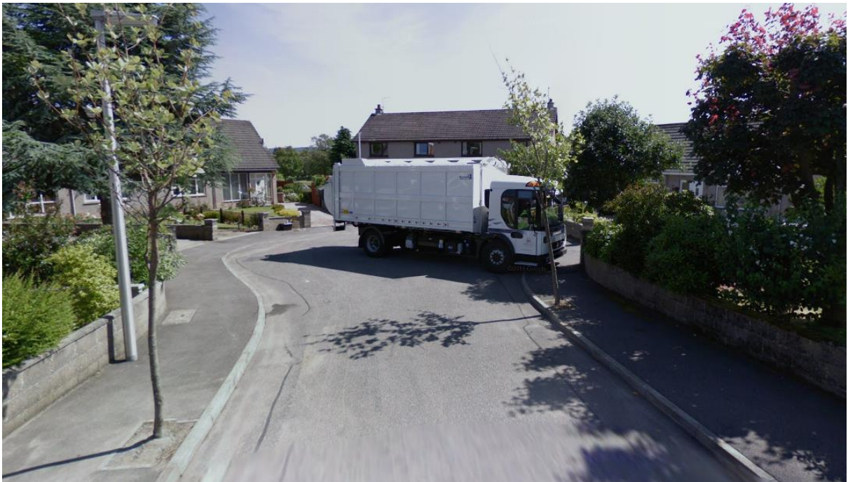
Example of refuse vehicle negotiating turning circle
